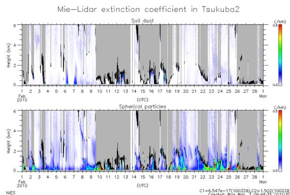
Figure 1: An example of final results of routine data reduction system. Dust extinction (top) and spherical particle extinction (bottom) at Tsukuba, Japan in February 2010. Black indicates cloud (between cloud base and apparent cloud top), and gray indicates areas where no data is obtained from lidar observation. This figure is made by post processing using one month data.
