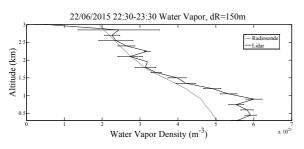
Figure 3. The 1 hour average water vapor density with 150 m range resolution and the radiosonde data.
