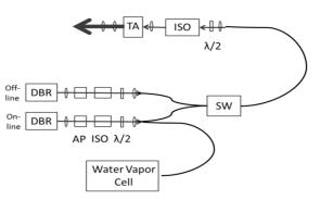
Figure 1. Block diagram of the DIAL transmitter.
