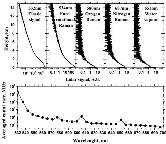
Figure1. Vertical profiles of elastic and Raman lidar signals (upper panels) and raw spectra (bottom panel) averaged across the vertical range from 100m to 2000m. Measurement time was from 1009-1057 UTC on 6 February 2009.
