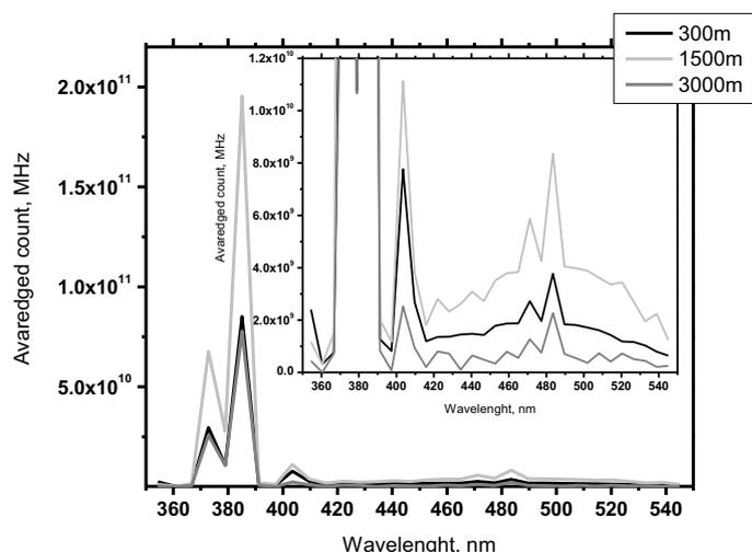
Figure 3. Raman and fluorescence spectrum at heights range 300m, 1500m and 3000 m. The measurement was carried out at Tsukuba from 15:00 to 19:00 UTC on 19 April 2010.
