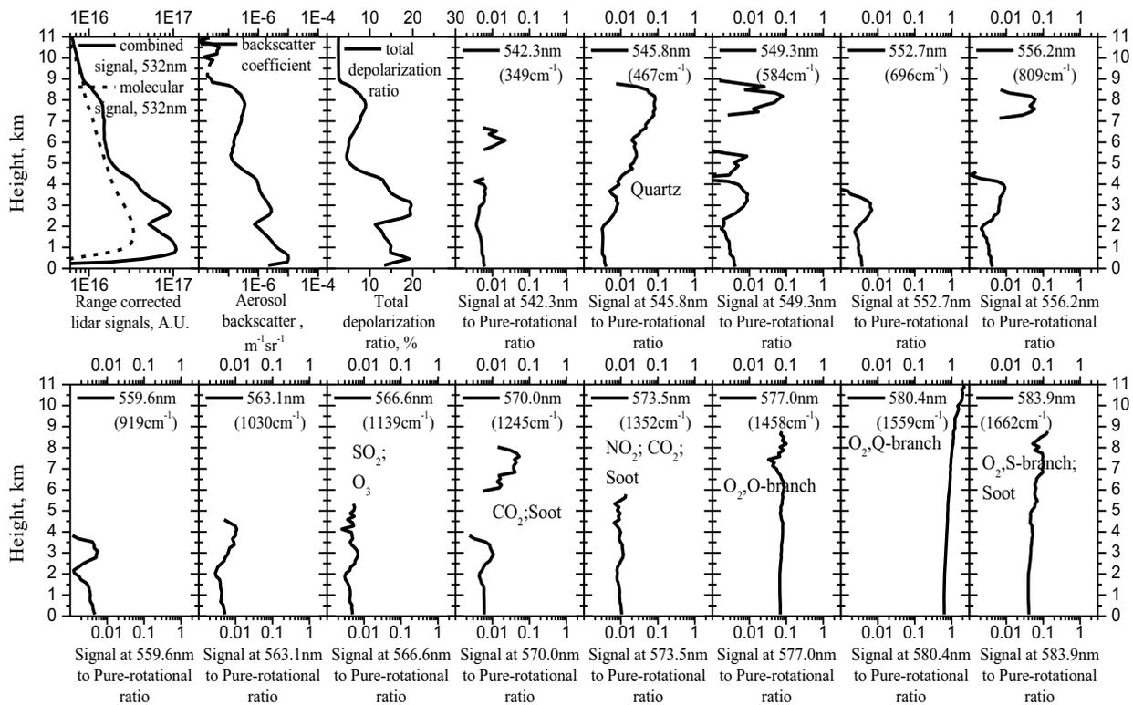
Figure 2. Vertical profiles of lidar return signals at different detection wavelengths during the advection of a mineral dust plume observed from 1105 to 1745 UTC on 17 March, 2009.
