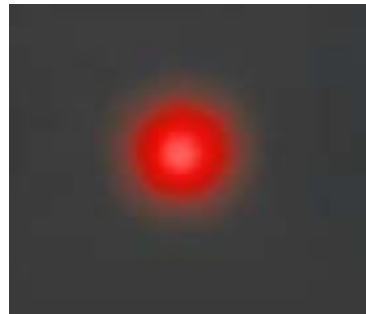
Fig. 3 Example of infrared LRNB generation. A semiconductor laser beam ( \lambda = 1.5 \mu\text{m} ) was transmitted by a 2.5cm diameter telescope. The picture of beam pattern was taken at 30m distance.
