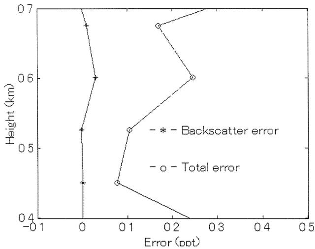
Fig.4: Backscatterer error and total measurement error
