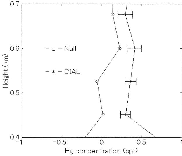
Fig.3: Null profile and Hg concentration profile with statistical error
