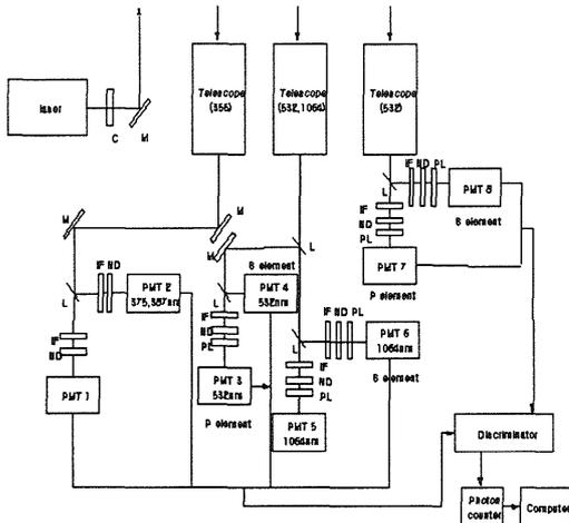
Figure 3. LIDAR Composition
