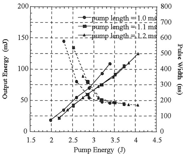
Figure 2. The output energy (solid line) and pulse width (dashed line) as a function of pump energy. The circles represents the temperature of the laser rod at 14 degree C for a pump duration of 1.0 ms. The squares and triangles represent the temperature of the laser rod at 19 degree C for the pump duration of 1.1 and 1.2 ms, respectively.
