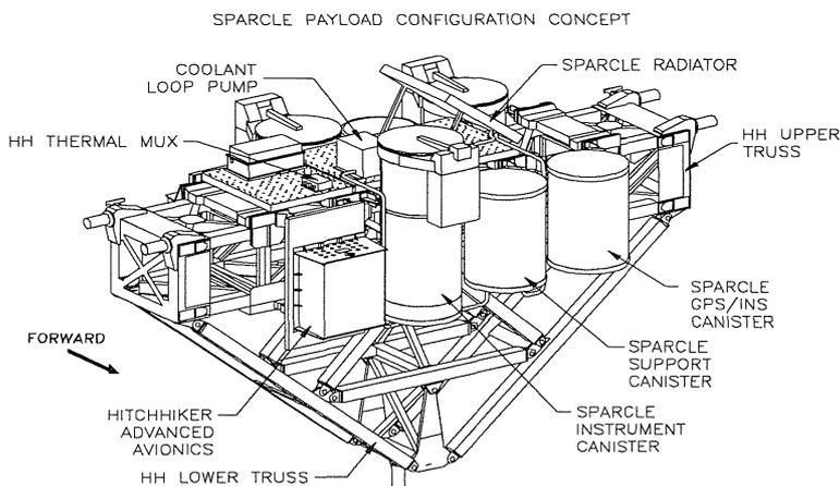
Figure 7. SPARCLE hardware configuration
