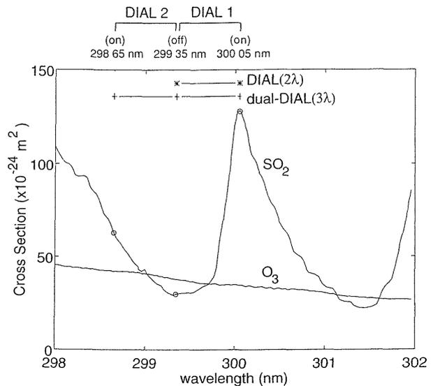
Fig. 3. Wavelengths used in 3-wavelength dual DIAL, and absorption cross section of  $SO_2$  and  $O_3$ .
