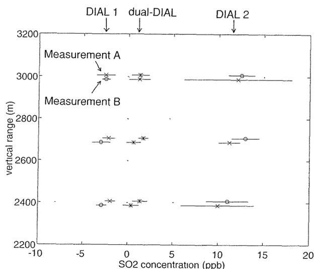
Fig. 4. Vertical SO<sub>2</sub> concentration profiles measured by 3-wavelength dual-DIAL. Profiles measured by only DIAL 1 or DIAL 2 are also indicated.
