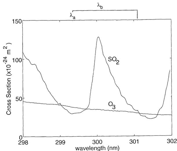
Fig. 1. Absorption cross section of  $SO_2$  and  $O_3$ , and wavelengths used in the  $SO_2$  measurement.
