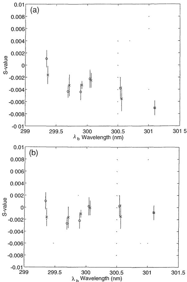
Fig. 2. Measurement results of  $SO_2$  concentration at 3300 m altitude.  $\lambda_a$  and  $\lambda_b$  are treated as *off* and *on* wavelengths, respectively. (a) S-value versus  $\lambda_b$ . (b) S-value versus  $\lambda_b$  after subtracting  $O_3$  contribution calculated from the  $O_3$  measurement data.
