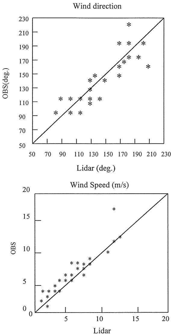
Fig. 2 A comparison of lidar and balloon wind measurement in Hong Kong (after Leung et al., 1995)
