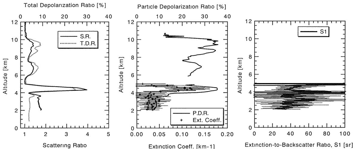
Figure 6. Mie-Raman lidar observation at TUMM/Tokyo on May 1st, 1999. The integration time is between 19:34-21:59 LT.
