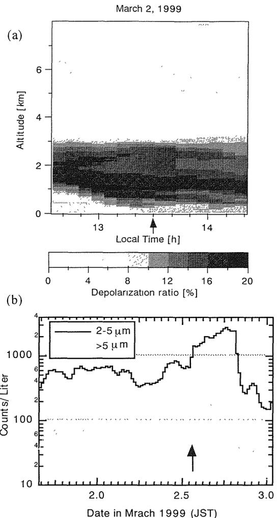
Figure 5. Descent of dust layer in the boundary layer on March 2, 1999 at Tokyo. Time series of (a) Lidar depolarization ratio vertical profile and (b) number of large particles counted by optical particle counter. The arrow indicates the time when the dust reached the ground level.
