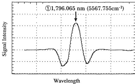
Fig.6 TDLAS Spectrum of H<sub>2</sub>O
