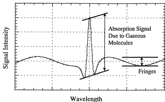
Fig.3 Absorption Signal Accompanied by Fringes
