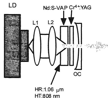
Fig. 1 Schematic diagram of the passively Q-switched Nd:S-VAP laser
