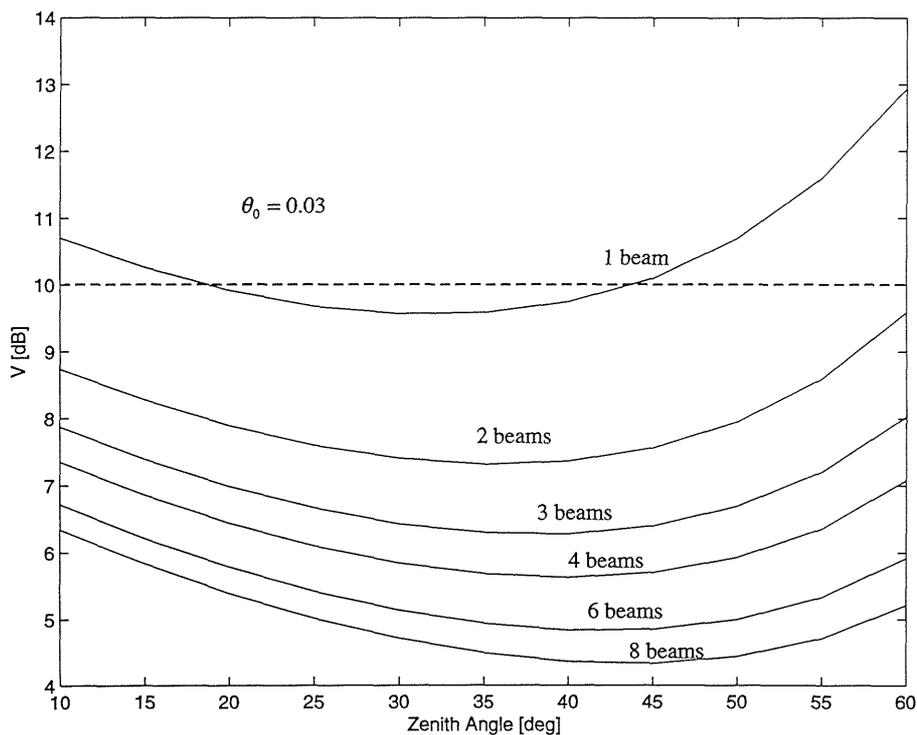
Figure 1. Received level variation at the OICETS satellite as a function of an elevation angle when assuming a fade probability of 1 % and a surge probability of 10 %. Transmitting beam divergence angle is 0.03 degrees (half angle).
