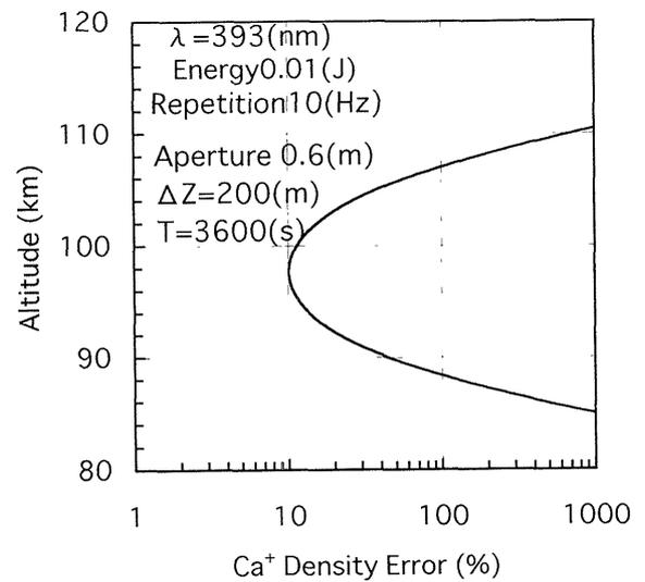
Figure 4. Calculated error of ionic calcium measurement.
