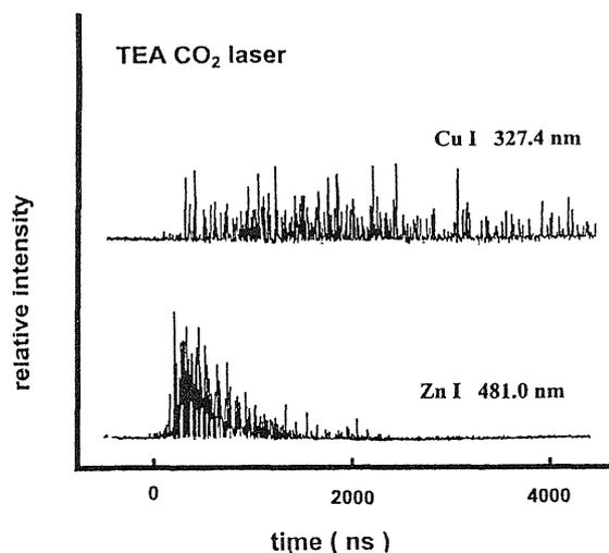
Fig. 3. Time-profile of the emission intensity of Cu I 327.4 nm and Zn I 481.0 nm using TEA CO<sub>2</sub> laser. Data was collected at 5 mm above the sample surface at a reduced pressure of 1 Torr.
