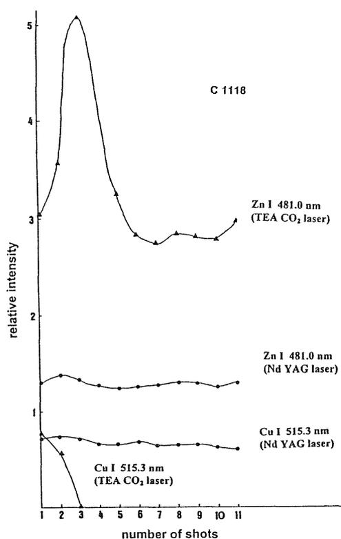
Fig. 2. Relationship between total emission intensity (time and spatially integrated) of Zn I 481.0 nm and Cu I 515.3 nm as a function of the number of shots of laser irradiation for TEA CO<sub>2</sub> laser and Nd-YAG laser
