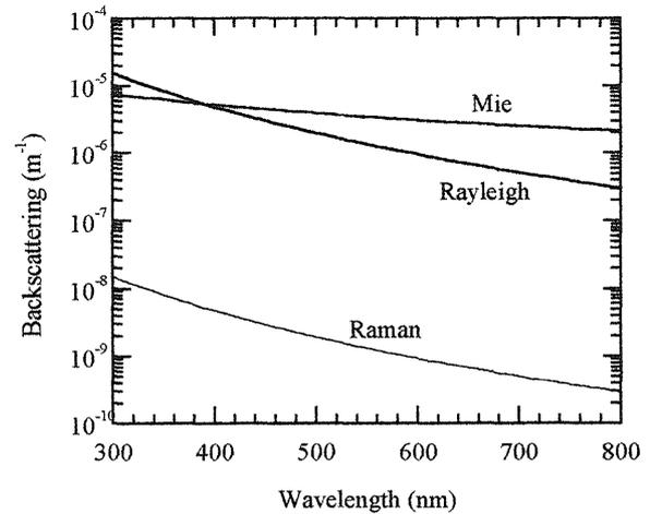
Fig.3 Backscattering coefficient vs laser wavelength
