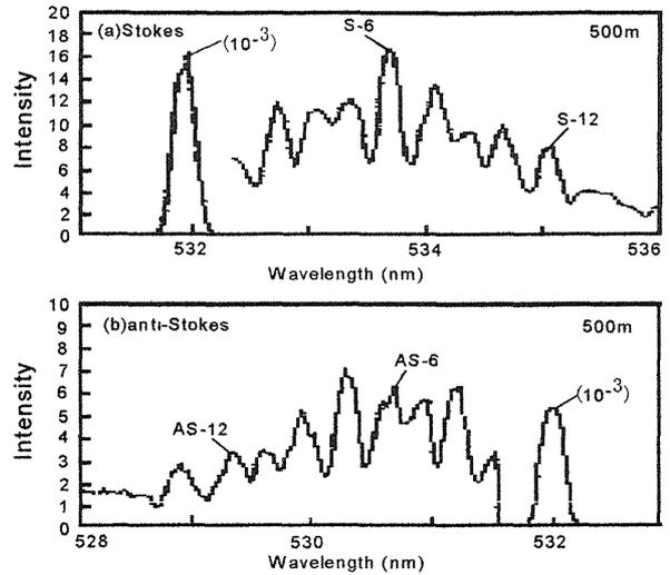
Fig.2 Rotational Raman spectrum with 532nm laser.
