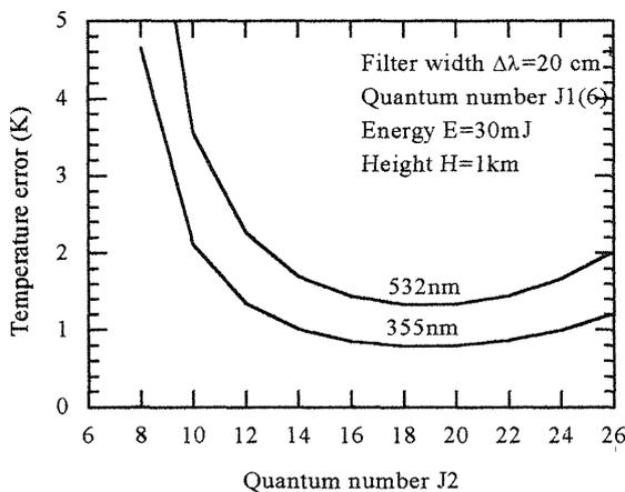
Fig.4 Temperature accuracy vs. anti-Stokes lines for 355nm and 532nm at the height of 1km.
