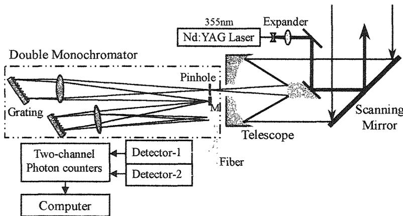
Fig.1 Schematic of UV rotational Raman lidar system
