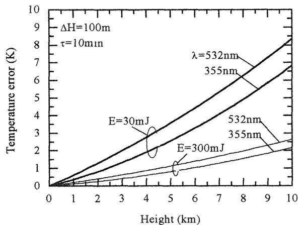
Fig.5 Temperature error vs height for 355nm and 532nm lidar systems.
