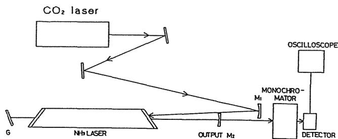
Fig.4 Experimental setup of NH<sub>3</sub> laser pumped with very high power CO<sub>2</sub> laser
