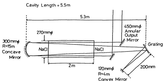
Fig.3 Experimental setup of very high power CO<sub>2</sub> laser
