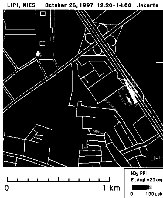
Fig. 9. Distribution of NO 2 measured with an azimuth scan with the DIAL.
